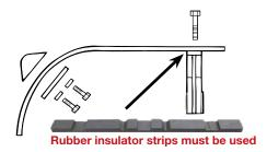
mate with the ribbed and smooth fender models. Round rubber grommets should not be used. The rear bracket must have a flat surface of 21" by 2" to properly secure the fender, and ensure maximum effectiveness and longevity of the fender.
